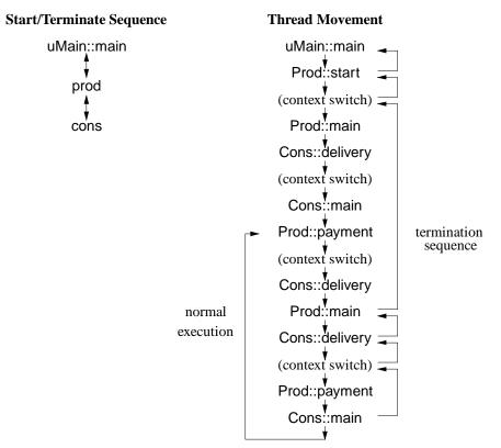
Figure 2.4: Cyclic Control Flow in Full Coroutine
