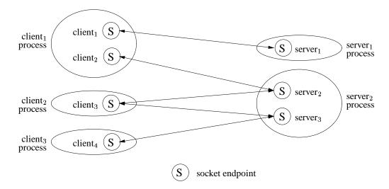
Figure 3.2: Client/Server Connectionless
